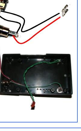
Bring the two halves together, taking care that the LEDs go into their holes.
