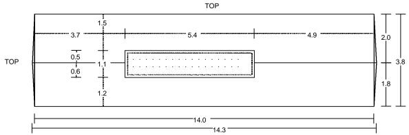
Cut the notch for the RS232 DB-9 connector on the right side of the top of the case.
