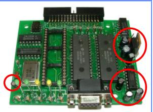
Mount the top six 10k (or 11k) pull-up resistors (R1-2, 8-11). Five are mounted above the memories and one to the left of the oscillator.
