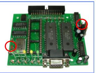
Insert the PIC (IC8) into the socket. Be VERY careful not to allow the pins to bend while inserting it.
