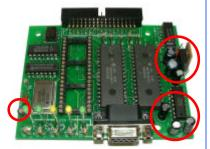
Mount the top six 10k (or 11k) pull-up resistors (R1-2, 8-11). Five are mounted above the memories and one to the left of the oscillator.
